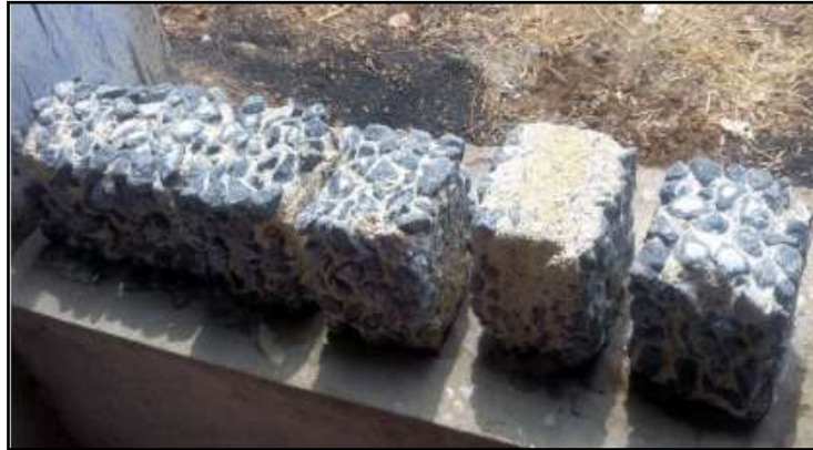
Figure 4.46 Concrete cubes after H 2 SO 4 exposure
