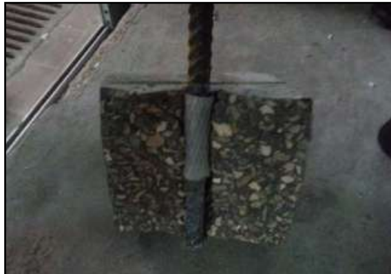
Figure-. 16 mm rebars splitting behavior.
